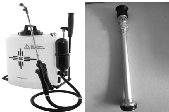
Figure 3. Knapsack sprayer equipped with a nozzle used for field application of the Bintaro fruit extract pesticide.
